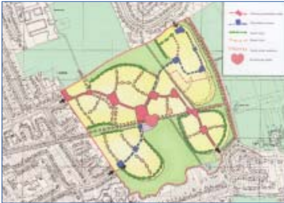
Pedestrian, cycle and bus routes designed at the start, New Osbaldwick, York (ref: PRP 2002)
